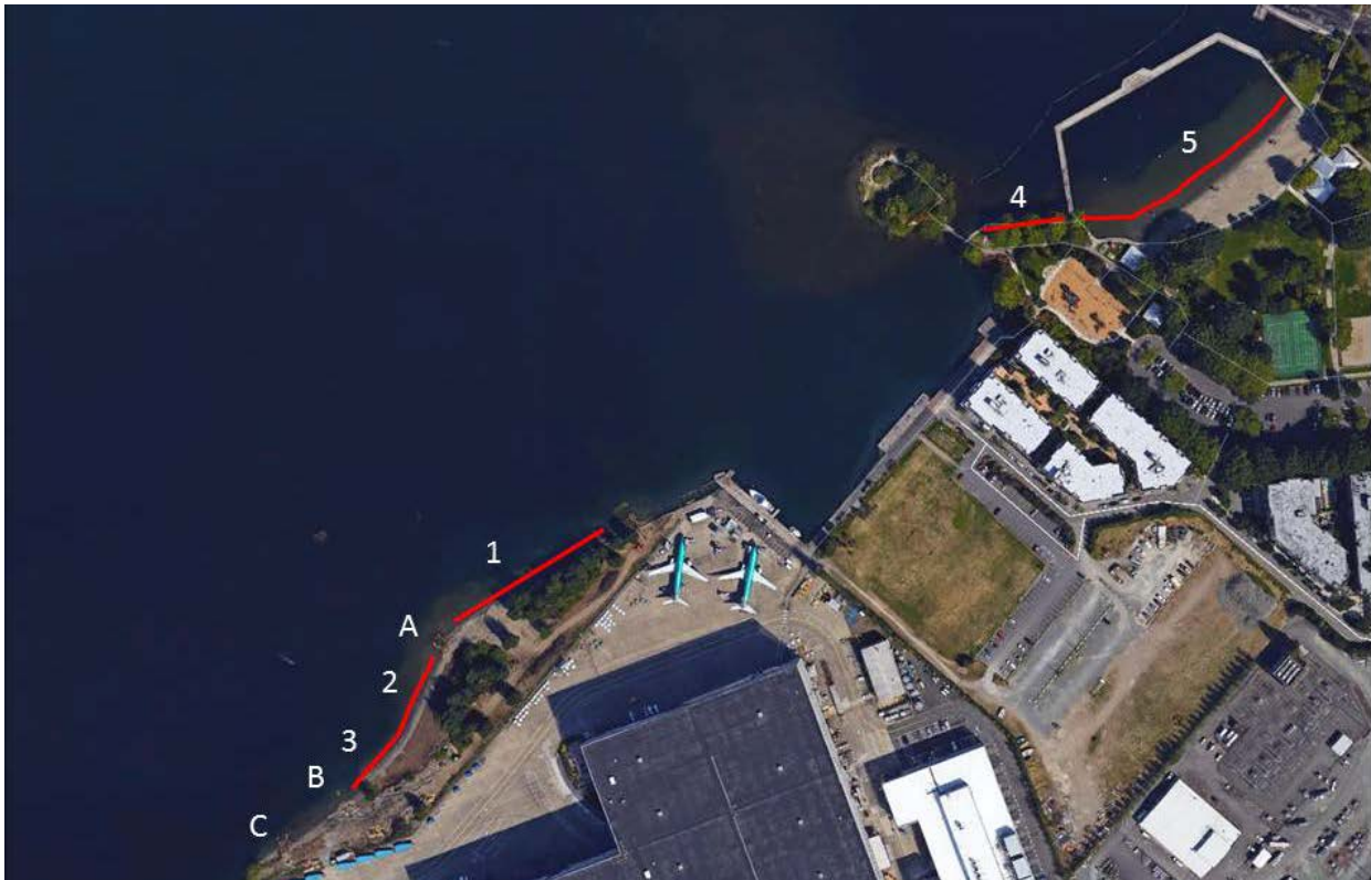
FIGURE 1.— Location of five transects (#'s 1-5) and three engineered log jams (A-C) used to monitor abundance of juvenile Chinook salmon in the south end of Lake Washington, January-June 2015. Transect numbers correspond to numbers in Table 1. The land adjacent to transect #'s 1-3 and engineered log jams A-C is WDNR property. The developed property to the southeast of WDNR property is The Boeing Company property. Transects #'s 4 and 5 are in City of Renton's Gene Coulon Park.
