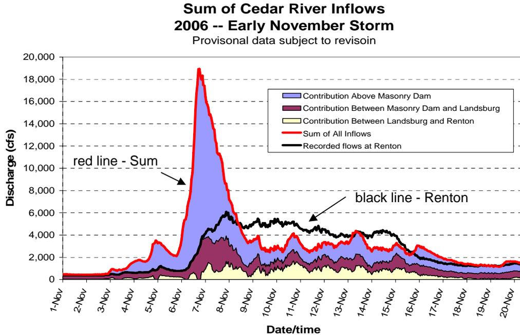
Figure 4. Cedar River November 2006 storm estimated inflow and discharge at Renton. Generally, the difference between the peak inflow (red line) and the actual discharge at Renton (black line) represents the reduction in flood magnitude due to storage at Chester Morse. The subsequent Cedar River flow at Renton (black line) that exceeds the inflow (red line) during the following days represents protracted flow duration. Figure provided by Seattle Public Utilities.
