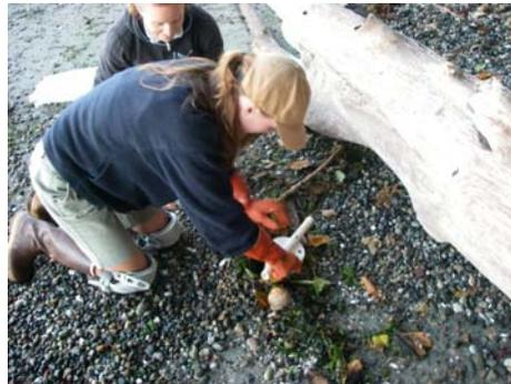
*A University of Washington student uses a length of PVC pipe to draw a core sample of the beach substrate at Seahurst this summer.*
